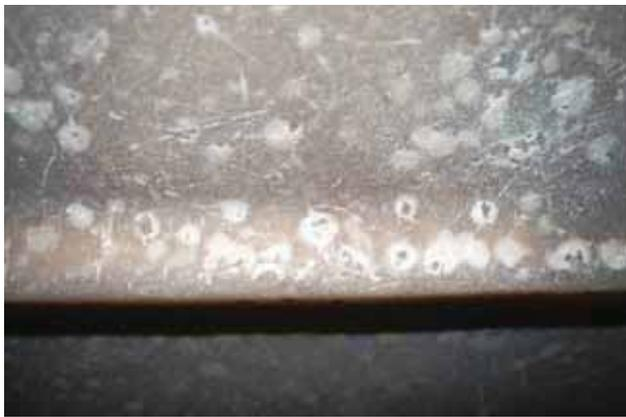
a 36 grade semi-rigid abrasive disc. This procedure replaces grit-blasting in the case of superficial osmosis, when removal the gel-coat layer is sufficient.
