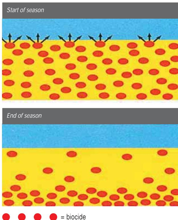
After some time, on the boat hull only the non active matrix is left. For this reason after the subsequent application of new antifouling, the thickness will increase. Therefore removal of the whole antifouling coat every 3 - 4 seasons is recommended. Hard antifouling should be preferred also for boats which are used daily as well as for boats used in brackish or fresh waters or in ports with strong currents.
