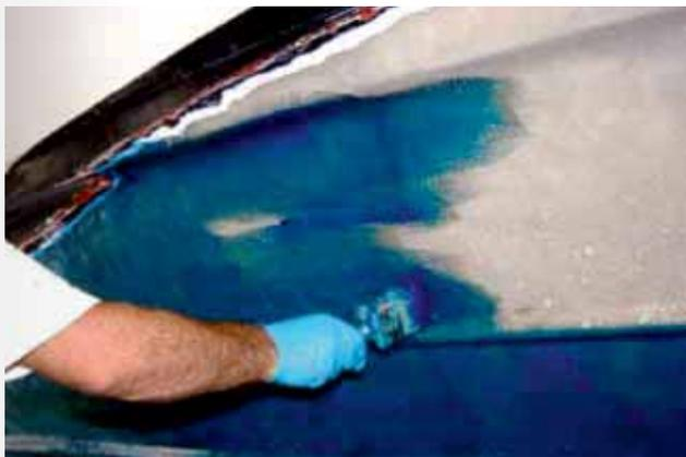
**7** After a drying interval of 16 hours minimum and 48 hours maximum (at 20° C), smooth all imperfections with the filler EPOMAST EVO, which has a low specific weight and therefore doesn't affect the weight of the boat significantly.
