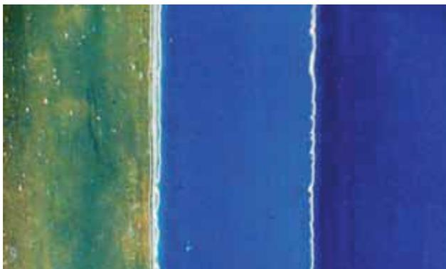
AQUASTOP should be applied within a temperature range of 15° to 35° C, at a relative humidity below 70% and with a humidity content of the boat hull not higher than 10%.
