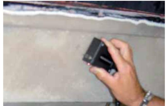
The hull can be considered dried out when the measured humidity content is below 10%.
