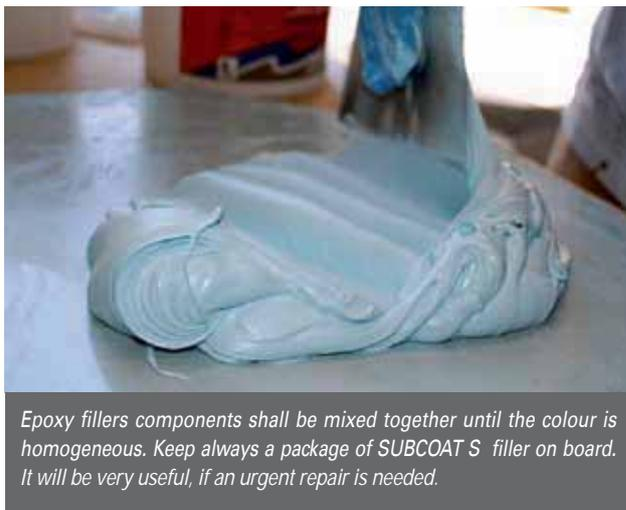
*Epoxy fillers components shall be mixed together until the colour is homogeneous. Keep always a package of SUBCOAT S filler on board. It will be very useful, if an urgent repair is needed.*
