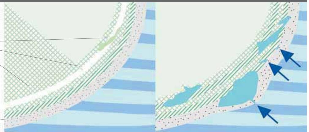
The diagram shows the resistance against water penetration for different materials used as barrier coats for boats.
